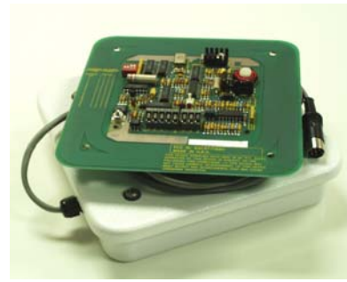
Model 1885E Combo Multiplex Reader/Read Head FCC Approved Addressable Approximate size is 8" x 8" x 1.5"
