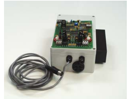
Model 1841E Dual Reader (handles 2 non-addressable Read Heads) FCC Approved Approximate size is 8" x 6" x 3"
