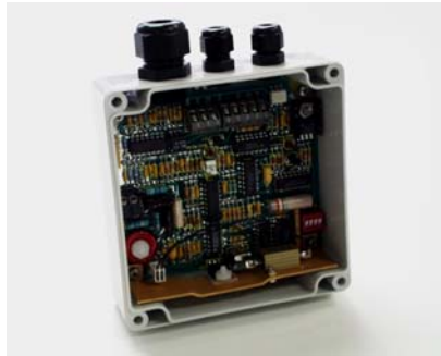
Model 1845E Multiplexing Reader FCC Approved Addressable Approximate size is 4.75" x 4.75" x 2"
