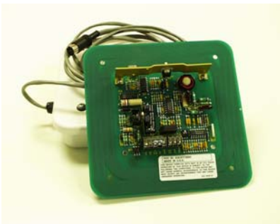
Model 1880E Combo Simplex Reader/Read Head FCC Approved Approximate size is 8" x 8" x 1.5"
