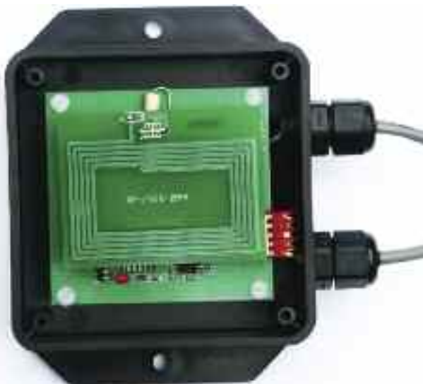
Reader Mounted in Housing (lid not shown)
